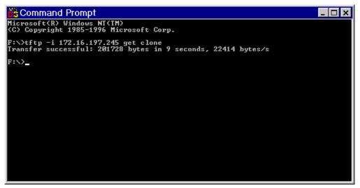
Figure 5.15: TFTP Protocol for Cloning a File
